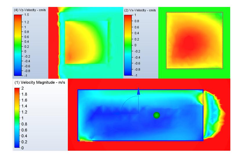
• Airflow Distribution: The aerodynamic effects inside the container indicated that the wind near the hodoscope exhibited fluctuations and lacked a stable pattern.
