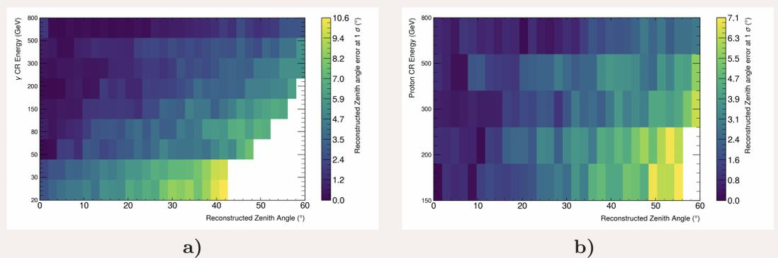
**Figure 4:** Heat map of angular reconstruction errors as a function of true zenith angle and primary particle energy: (a) Photon as CR (B) Proton as CR.
