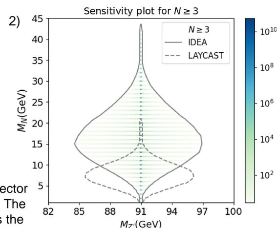
Fig.3: Displaced activity on a far detector that consists of a one-layer tracker. The color bar on the right plot represents the number of expected events.
